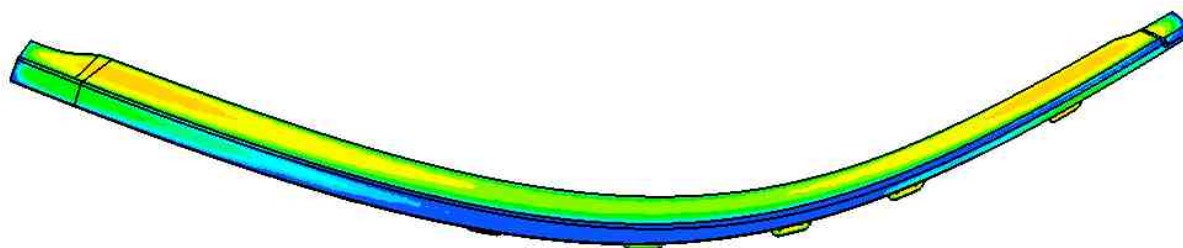
Fig. 1: Simulated Cr deposit layer thickness on a single part
