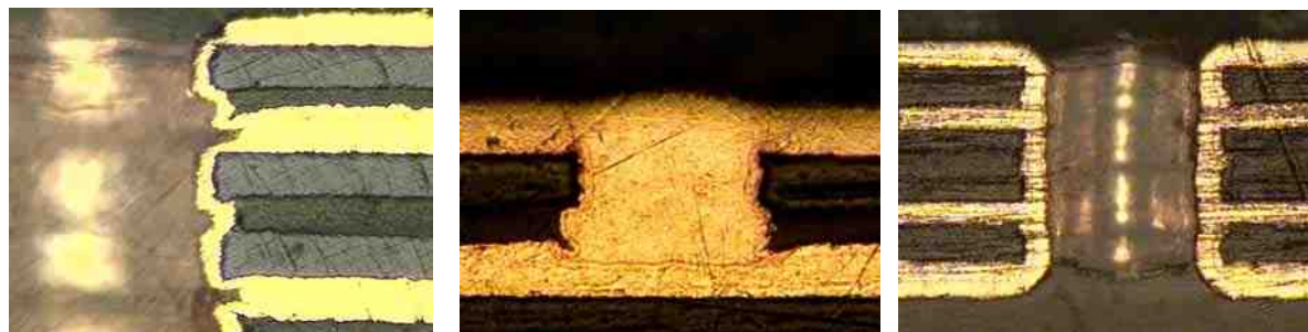
Figure 9. Multilayered PI-flex: Envision HDI-Flex Initiator 7325 & Envision HDI Catalyst 7375 treatment prior to Cuprostar® C VF1 flash (upper left) followed by 100% microvia fill (middle) and 100% PTH (right).
