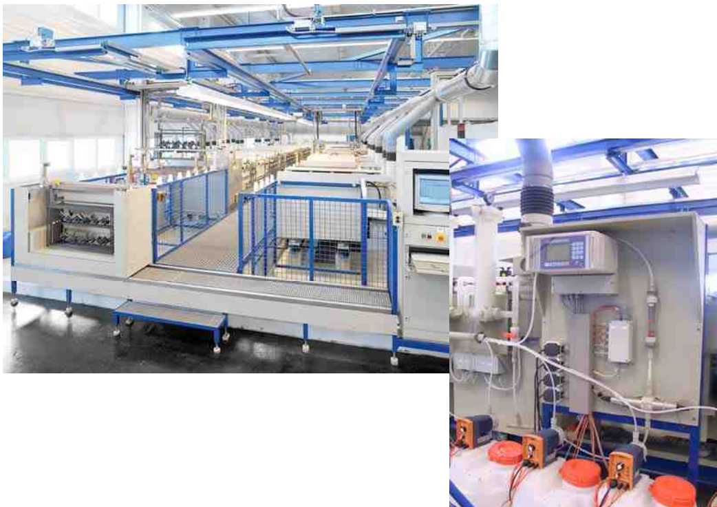
Figure 7: Automatic Metallizing Equipment for MIDs with Online-Analytical Controls (I&T AG, Austria)
