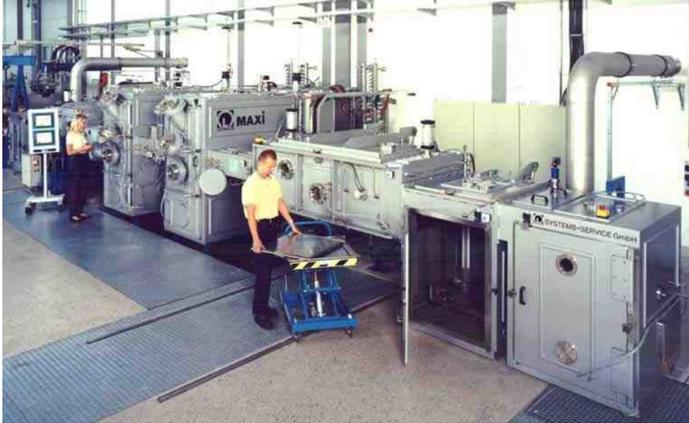
*Figure 7: In-line PVD coating plant MAXI*
