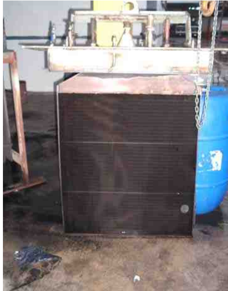
Photograph 4.- View of a completely corroded anode electrode.
