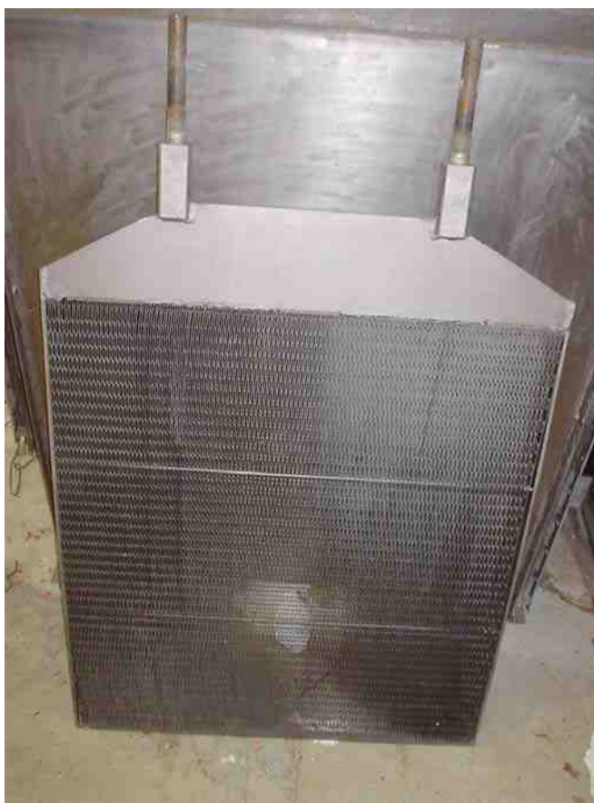
Photograph 9.- Electroless nickel plated anode electrode.
