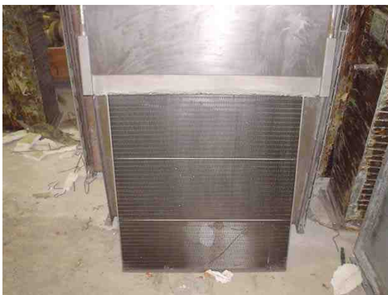
Photograph 10.- Electroless nickel plated cathode electrode.
