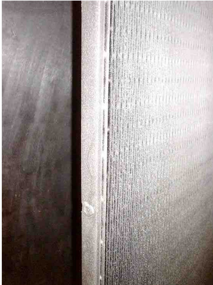
Photograph 11.- Corrosion pits protected against corrosion with electroless nickel.
