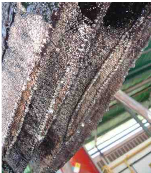
Photograph 3.- Detail of the cloth bags that cover the anode and cathode electrodes.
