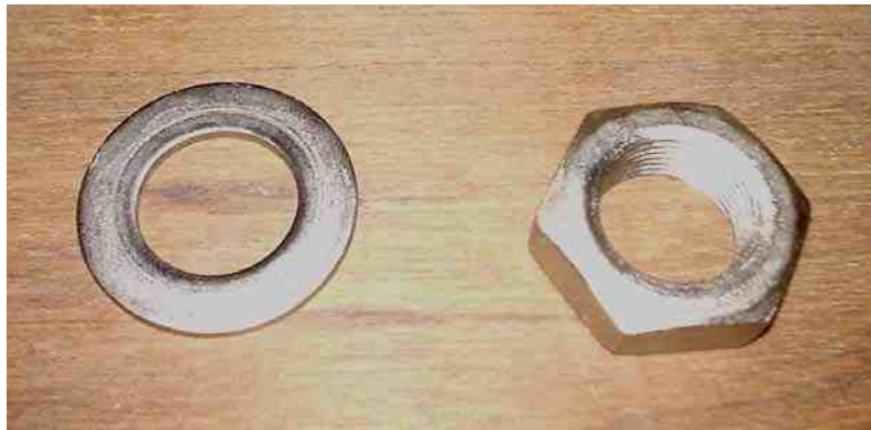
Photograph 7.- Electroless nickel plated Fasteners.
