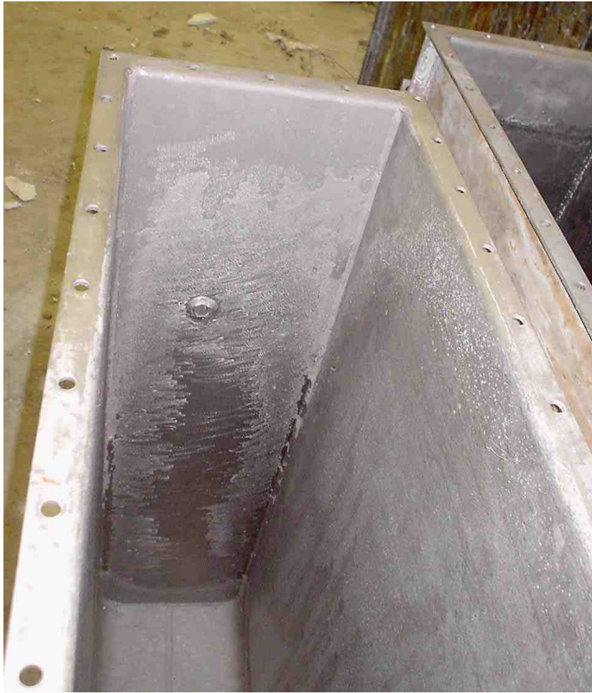
Photograph 8.- Electroless nickel plated cell box.
