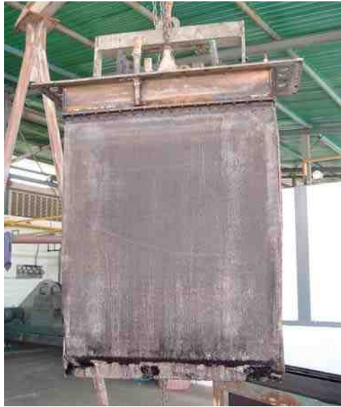
Photograph 2.- A view of the tank cover to which the anode and cathode electrodes are fastened.
