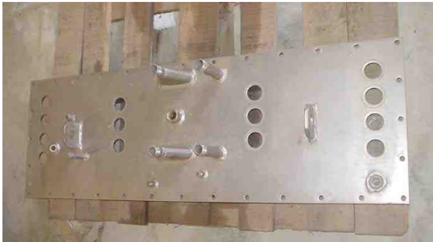
Photograph 6.- Electroless nickel plated tank cover.
