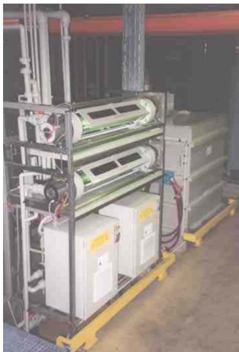
Picture 1: Typical Enviolet® UV System for Plating Bath Maintenance
