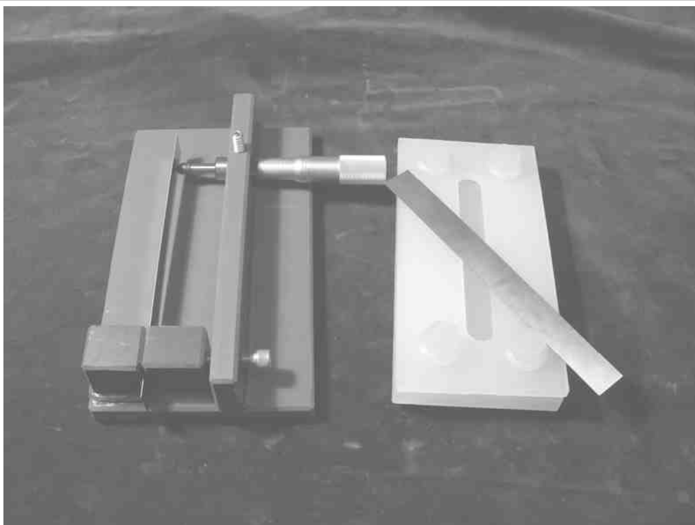
Figure 2 Bartlett Stress Strip Equipment
