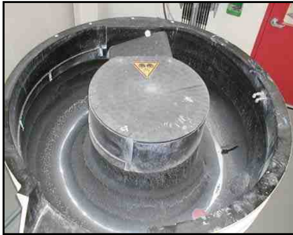
Image 1; Image shows an overhead view of a traditional vibratory bowl showing the toroidal shape of the bowl's operating channel. 2
