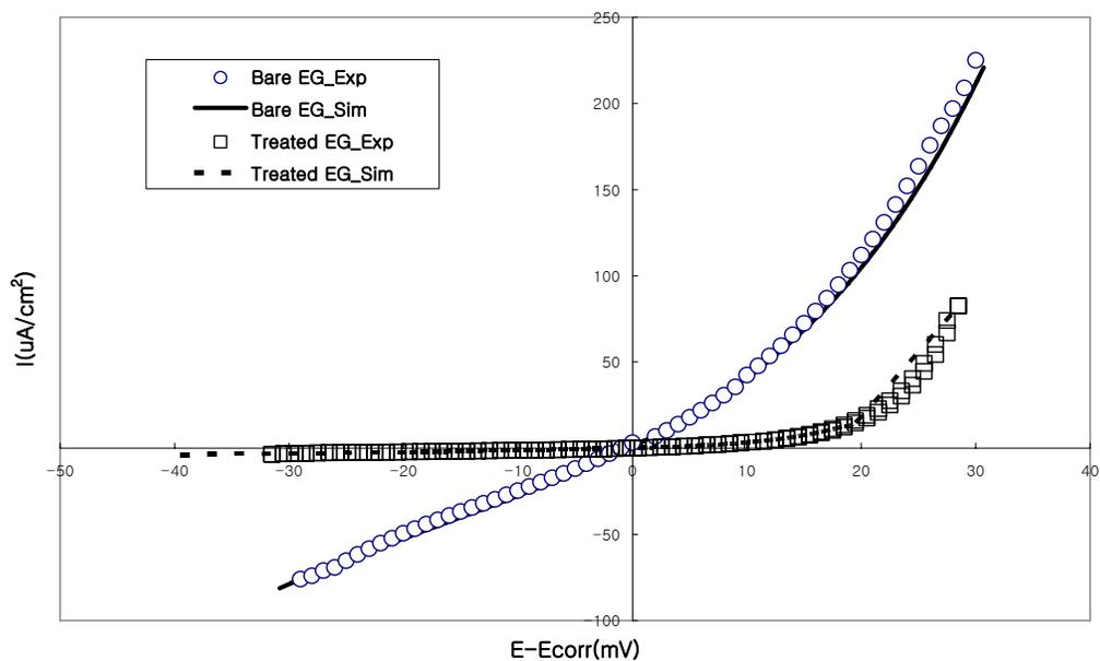
Fig. 1. Polarization curves for bare EG and treated EG exposed to 0.5N NaCl for 1 day
