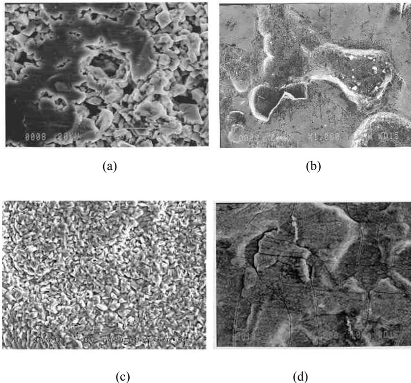
Fig. 3. SEM morphologies for bare EG(a), EN(b), GI(c) and GA(d)
