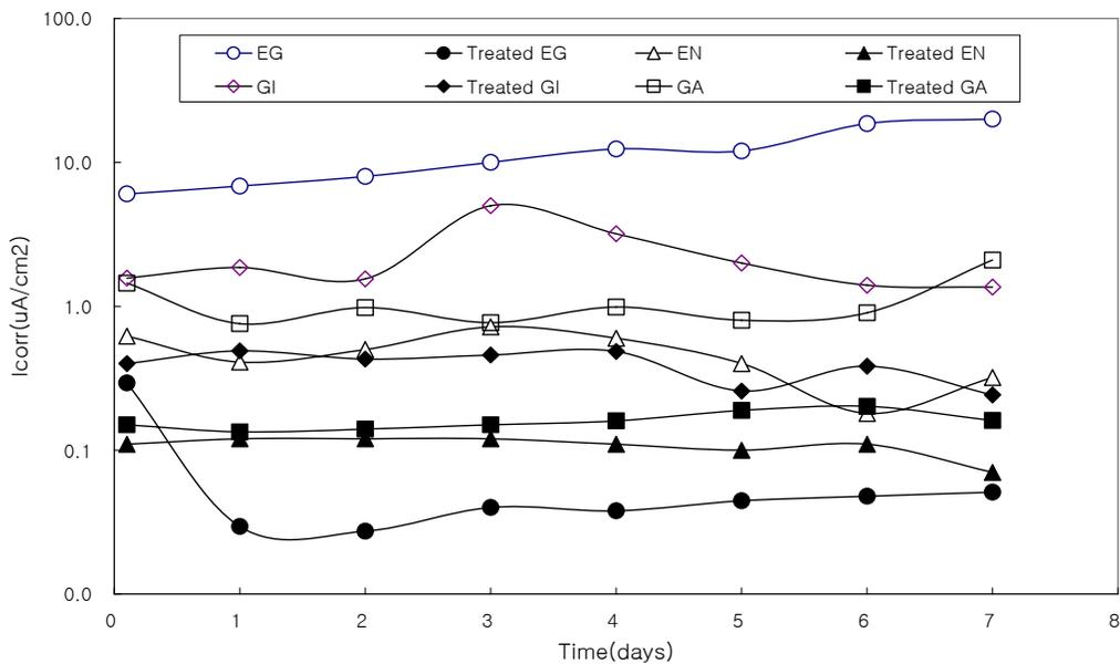
Fig. 2. Time dependence of  $i_{corr}$  for bare and treated samples exposed to 0.5N NaCl
