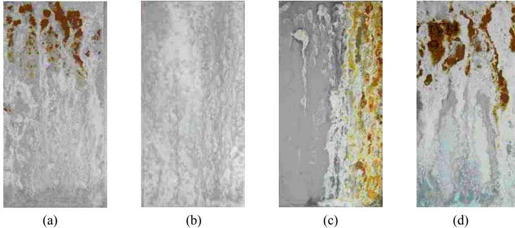
*Fig. 5. Salt spray results for treated EG(a), treated EN(b), treated GI(c) and treated GA(d) for 200 hrs*
