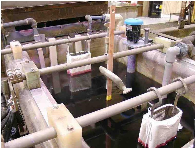
**Figure 7** 1500 L (~400 gal) nCoP Plating tank installed at NADEP-JAX.
