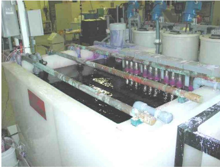
**Figure 6** 1200 L (~300 gal) nCoP Plating tank installed at Integran Technologies.
