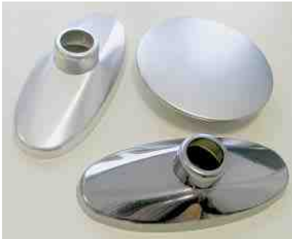
Figure 6: Satin matte parts plated with matte copper, bronze, and trivalent chromium in comparison with a bright part.
