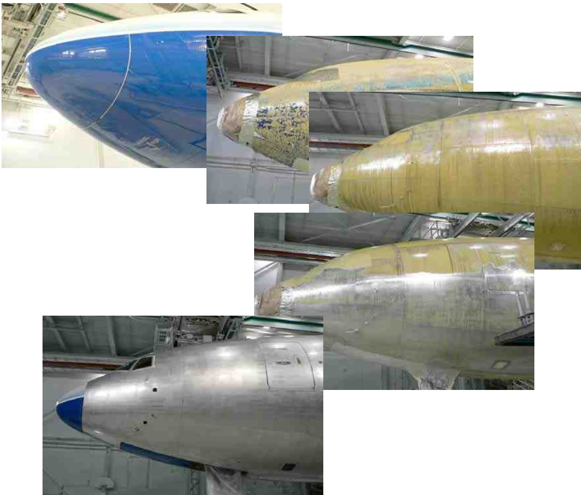
Figure 12 - Paint stripping sequence and complete coating removal from the sol-gel treated metal surface.
