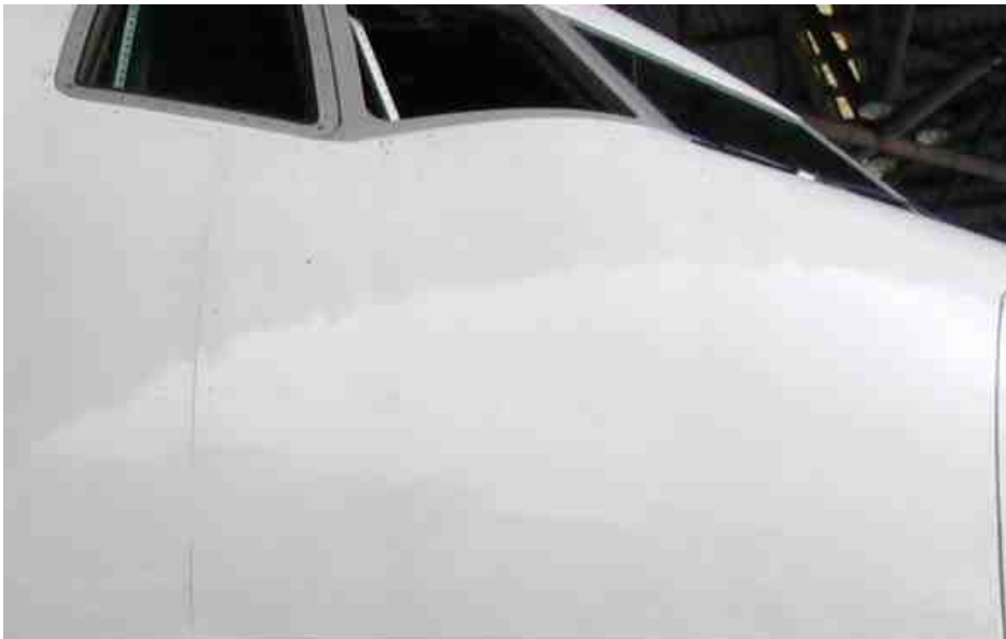
Figure 10 - Minimal rivet rash on a Boeing 777 painted after sol-gel rivet conversion after 14 months in-service.
