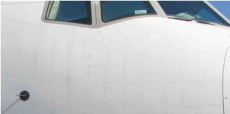
Figure 9 - Rivet rash on a Boeing 777 painted prior to sol-gel rivet conversion after 18 months in-service.
