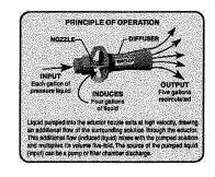
along the pipe to direct solution across the bottom or sides of a tank and into the recesses of the parts to replenish electrolyte.
