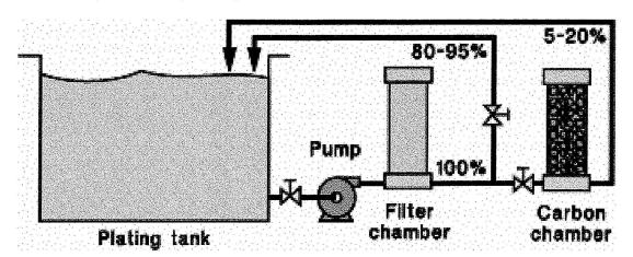
The choice of purification method depends on tank size, amount of carbon required, and other filtration equipment which may be available. Generally, carbon cartridges are used on tanks up to a few hundred gallons; bulk or canister type granular carbon is used for tanks of several thousand gallons. Granular carbon is also used as a separate purification system on the larger tanks to supplement surface filters, depth cartridges or certain
