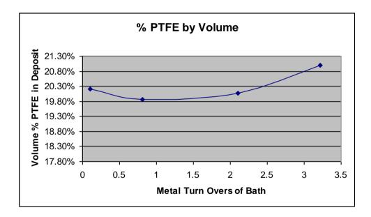
The trial work was done with a commonly used concentration of six grams per liter of PTFE dispersion in the plating bath. As is known in the industry, the percentage of PTFE in the deposit can be readily increased by increasing the concentration of PTFE dispersion in the bath. This was confirmed in the new system in additional trials where greater than twenty-five percent by volume PTFE was achieved by a relatively small increase in PTFE concentration in the plating bath.
