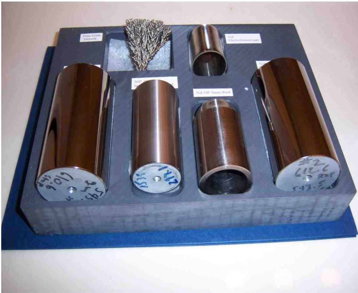
Figure 4 Electroplated NiP and NiCoP Samples Including 0.6 cm Thick Electroform
