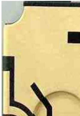
Fig. 10 Detail of SPS/SPS 2 shot part plated with ECu HS, Ni, Au in barrel
