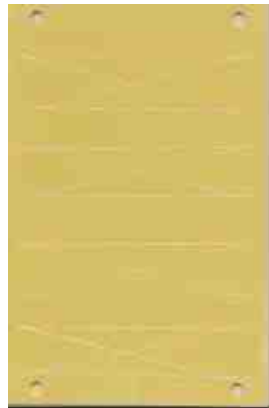
Electroplated Al with MIL-PRF-23377, after 7 days
