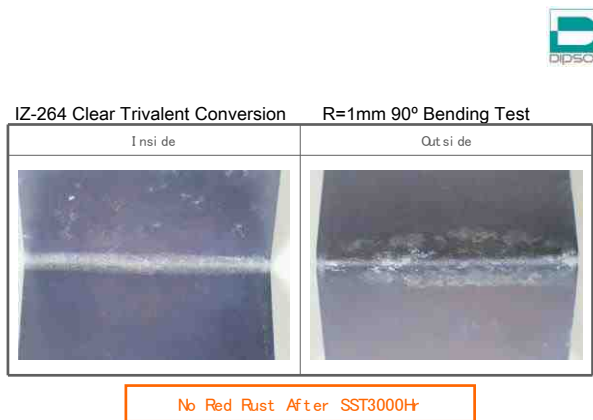
Fig-7) Bend test 3000hours after NSS
