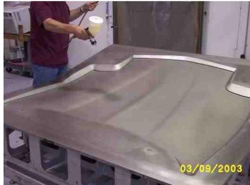
Fig. 1 Invar tool for Corvette carbon fiber hood outer production
