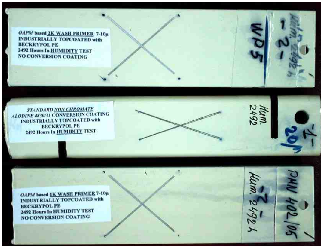
Figure 2: Al 6023 profiles after 2492 hours in Humidity test
