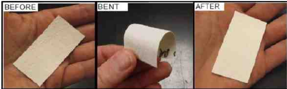
Figure 2 - Photographs of ceramic coated (Mylar®) flexible substrate showing no cracking or delamination during 180° bending.
