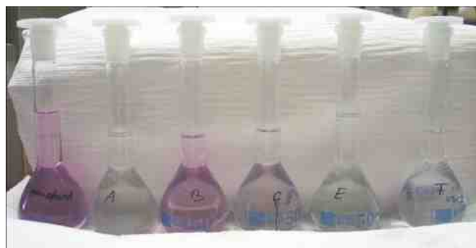
Figure 7 - Test according ISO 3613: 13 (L) = Reference solution; (A) = Cobalt-free passivate; (B) = Cobalt-containing passivate I; (C) = Cobalt-containing passivate II; (E) = Cobalt-free passivate after three months storage; (F) = Cobalt-free passivate after one week storage.
