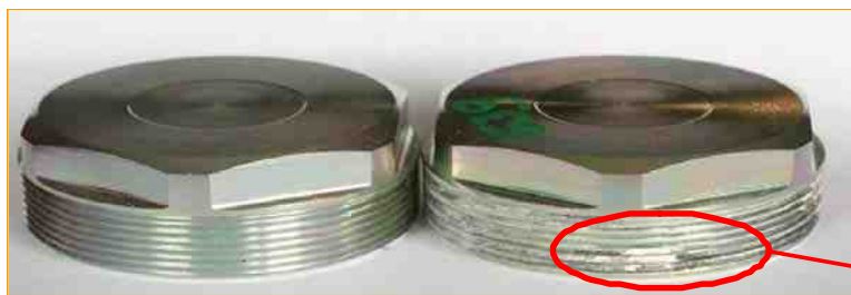
Figure 5 - Caps after 240 hr NSS: (L) cobalt-containing passivate; (R) cobalt-free passivate.
