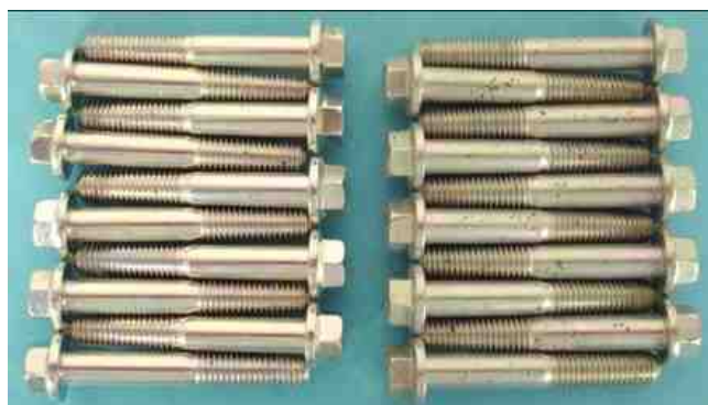
Figure 2 - (L) Fasteners with cobalt-free passivate; (R) fasteners with cobalt-containing passivate (both after 240 hr NSS).
