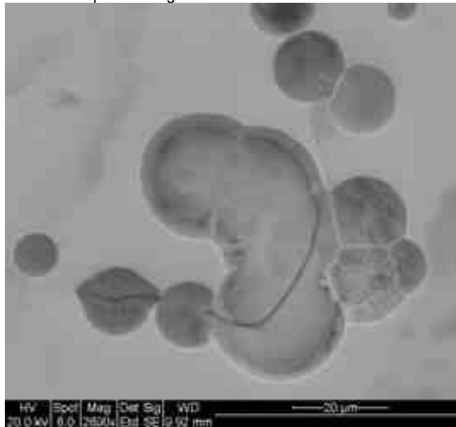
Figure 7 - Surface photo of duplex coating after 320°C heat treatment and 340 hr in neutral salt spray.
