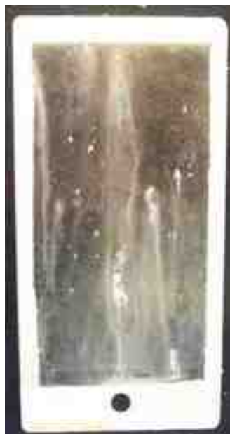
Figure 9 - Duplex panel of low-phosphorus upper layer and ternary alloy lower layer - as-plated after 894 hr in neutral salt spray.
