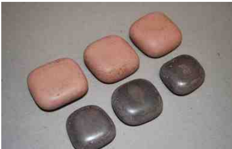
Figure 4 - Three pieces of high-density glazed media in the foreground compared to three pieces of clean media to the rear.
