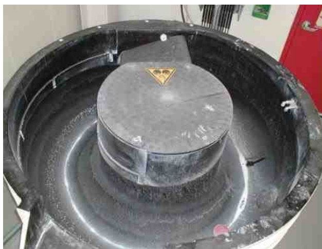
Figure 1 - An overhead view of a traditional vibratory bowl showing the toroid-shaped processing channel.
