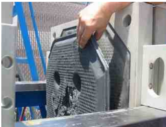
Figure 10 - The typical appearance of a 35 wt% solids filter cake generated in a filter press.
