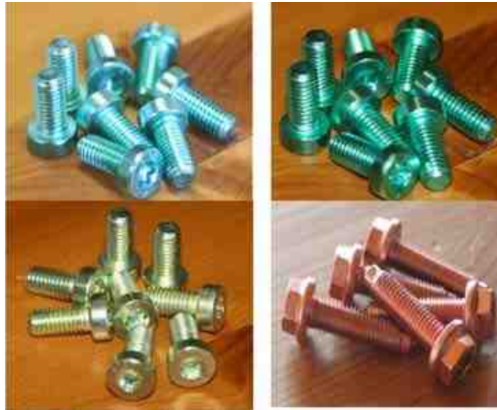
Figure 6 - Different colors produced on the passivates by dyeing.
