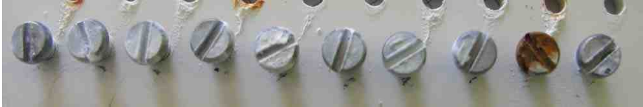
Figure 5 - Results of the salt spray test after 1800 hr for the screws from Fig. 4 (R).
