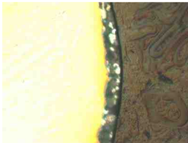
Figure 2 - Cross section of a part; (L) basis material, middle = zinc + nano-coating; (R) embedding material (The black line between the zinc and the embedding material is the nano-coating.).
