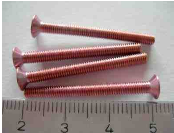
Figure 3 - Screws, zinc plated, clear passivate and a red dyed nano-coating.
