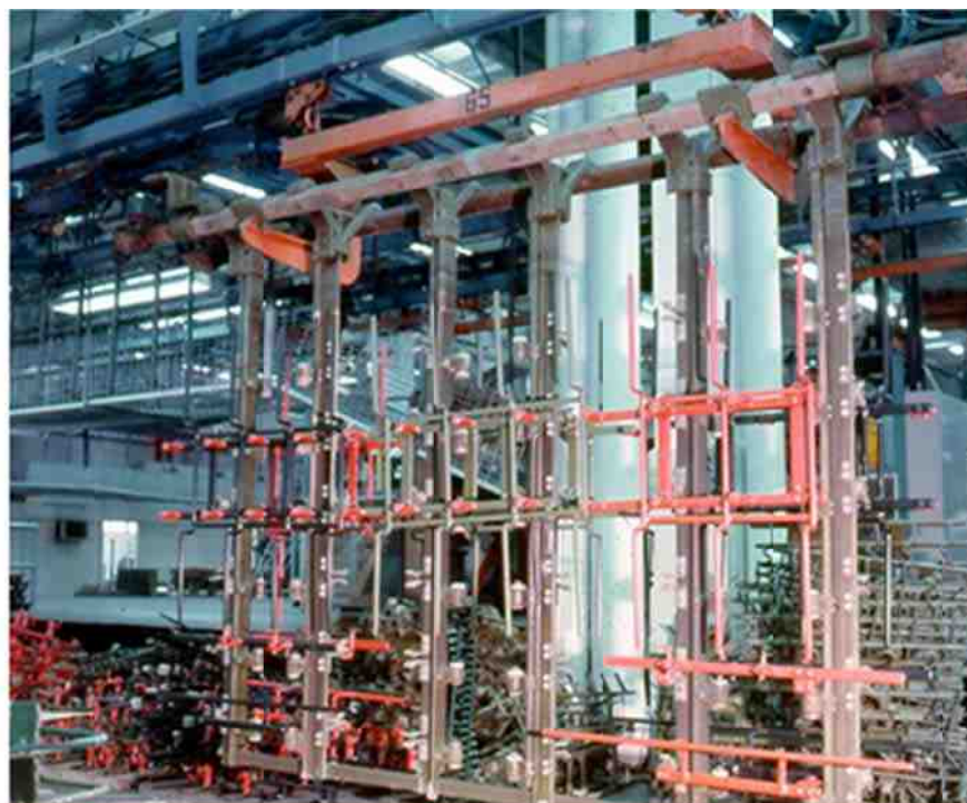
Close-up of large hoist rack for copper-nickel-chromium, including auxiliary anodes built into structure.
