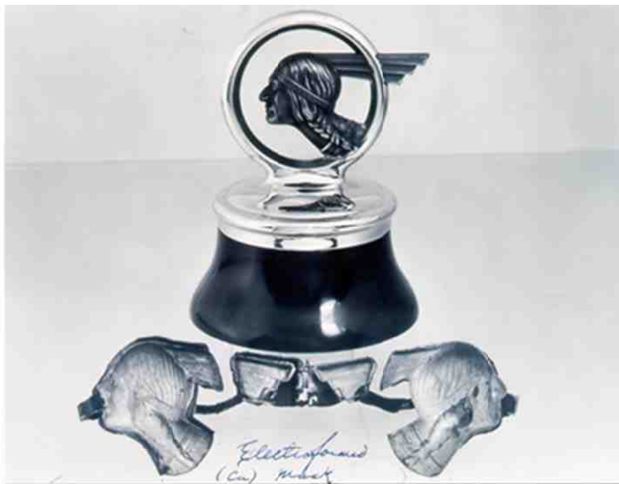
Art in Metal Finishing – A 1930s vintage Pontiac Indian Head radiator Cap. The base is electroformed in copper, bronzed and assembled to the chromium finished die-cast ring and cap piece.
