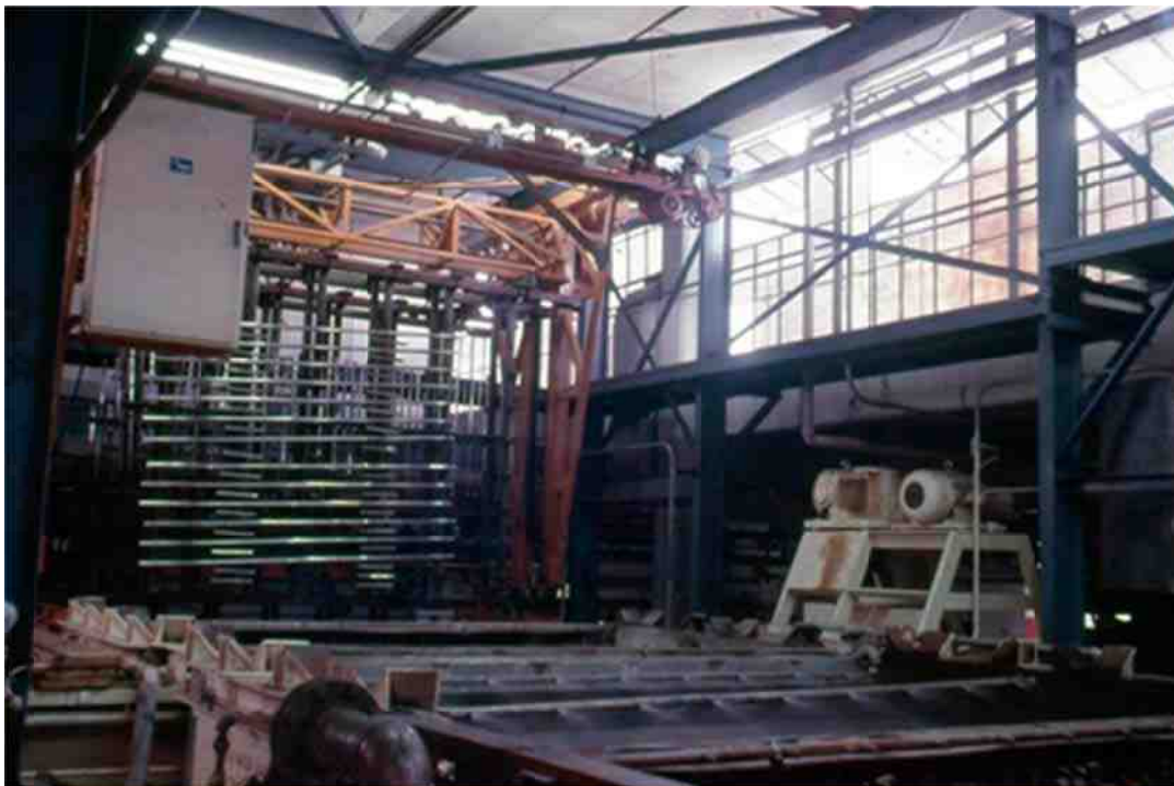
A massive hoist transfers a load of body side moldings to the next tank in the line.
