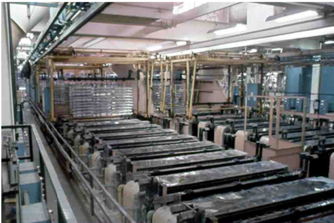
Another view of the copper plating side of the hoist line and the exhaust ducts between each station.
