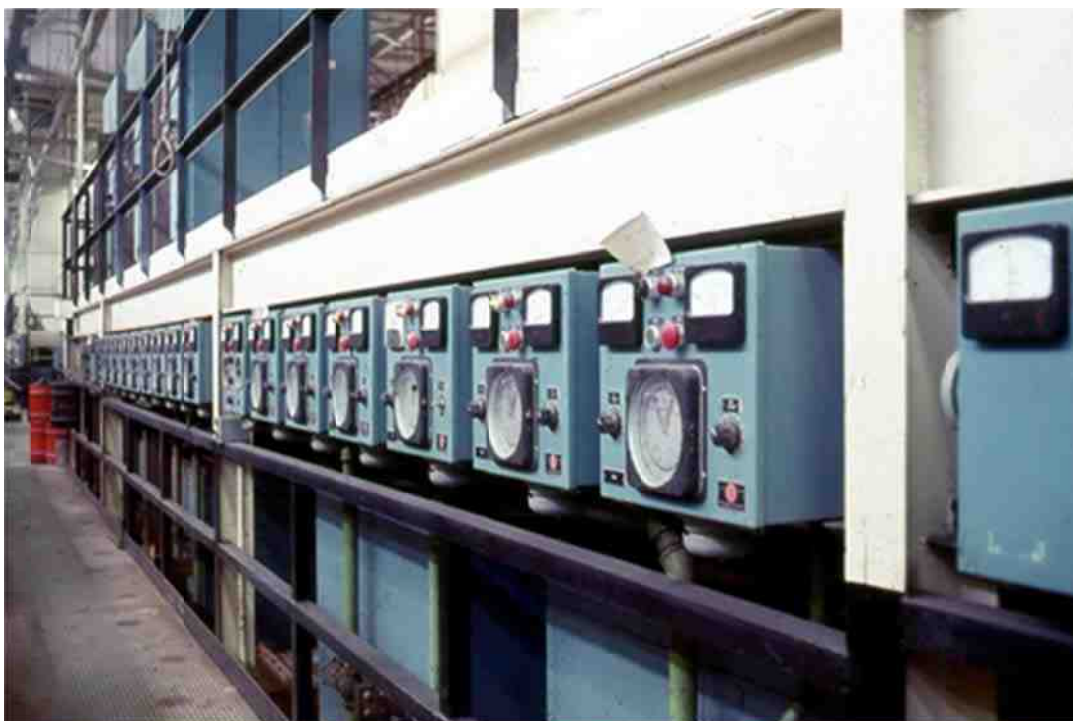
Periodic reverse controller for individual stations in the cyanide copper plating process.
