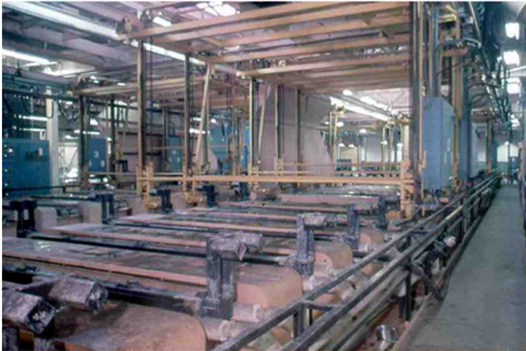
Looking down the copper plating side of the hoist line. Note the PVC exhaust ducts between each station.
