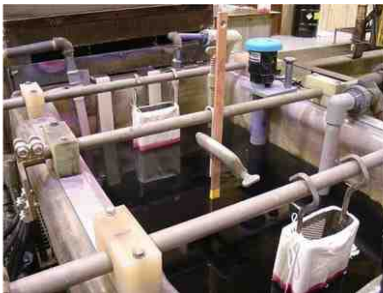
Figure 6 - Photograph of 300 gallon nCoP plating tank at FRCSE.
