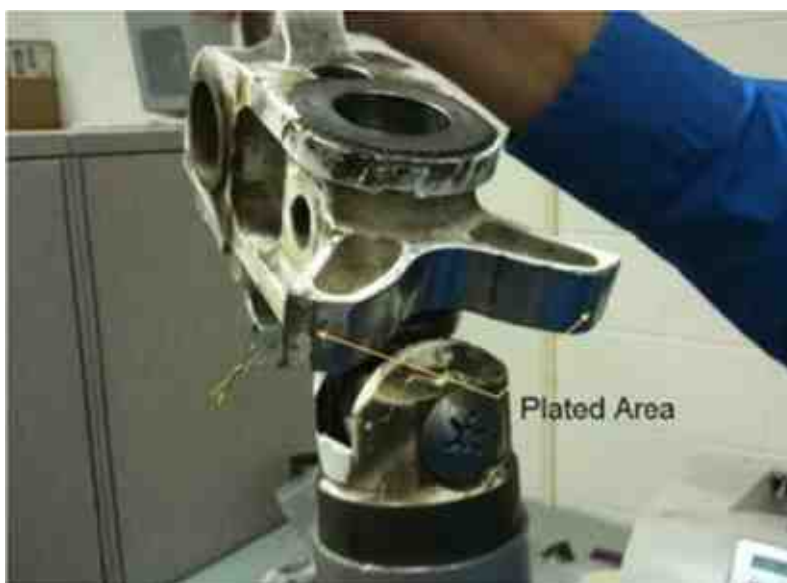
Figure 12 - Disassembled pivot assembly showing area on cam surface currently nickel and EHC-plated for wear resistance and proposed for nCoP plating.
