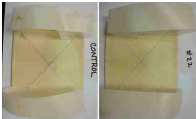
Figure 3 - Wet tape test results for non-chromated epoxy primed and scribed AZ31B-H24 magnesium alloys; bare (L), trivalent chromium-coated (R) magnesium samples. Scale from the surface was removed chemically. Trivalent chromium-based chem film on the magnesium alloy surface provided excellent tape adhesion characteristics with a rating of 5A in accordance with ASTM D3359 - Method A.
