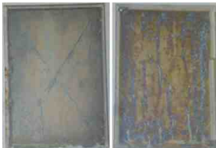
Figure 4 - Zn-Ni plated 4130 steel test panels sealed with the novel trivalent chromium (L) and hexavalent chromate (R) after 528 hr neutral salt fog test per ASTM B117.
