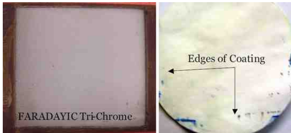
Figure 9 - Ferrocyanide test results for our trivalent chromium coating.
