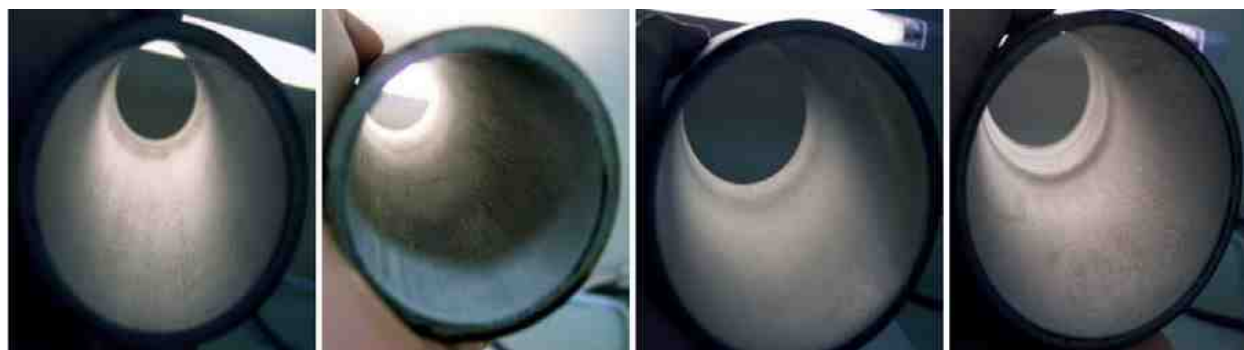
Figure 6 - Process scalability study: 4130 steel pipes coated with chromium at IDs/lengths of (a) 1½ × 6 in., (b) 1½ × 8 in., (c) 3 × 6 in. and (d) 3 × 8 in.
