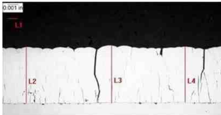
Figure 10 - Bend-to-break adhesion test results per AMS 2460, showing a direct comparison between the adhesion of trivalent chromium coating and a conventional hexavalent chromium coating.
