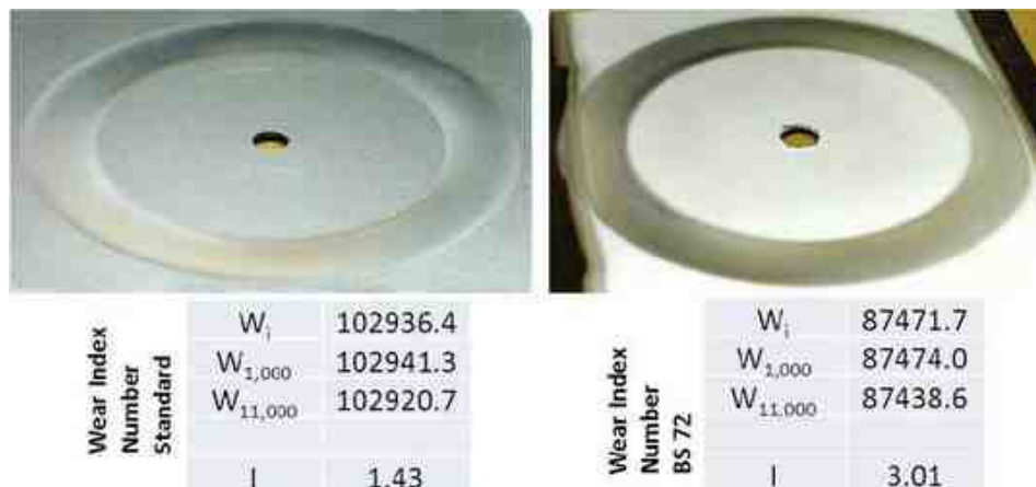
Figure 12 - Comparison of wear index numbers and Taber abrasion results for (left) hexavalent and (right) trivalent chromium plated samples.
