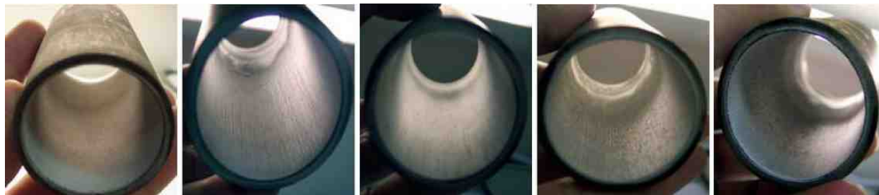
Figure 5 - Processing condition frequency optimization study: 1½ in. ID × 4 in. long pipes coated with chromium at a current density of 35 A/dm 2 and the frequency increasing from left (DC) to right (1000 Hz).
