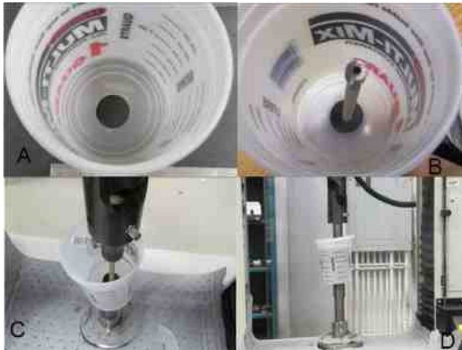
Figure 4 - Geometry 1a.1 and 1a.2: (A) the empty container, (B) the sample in the cup, (C) the sample loaded onto the mechanical test frame and (D) the sample being tested in solution.
