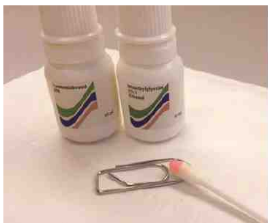
Figure 2 - A bright nickel plated paper clip reacting positive (red complex on the swab) on the dimethylglyoxime test (DMG).
