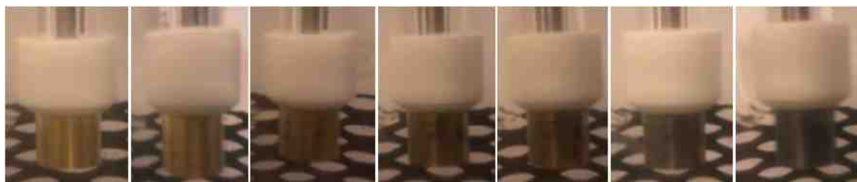
Figure 8 - Photo series showing how the gold layer is stripped from the tin/nickel coating over time during the anodic polarization of the working electrode.
