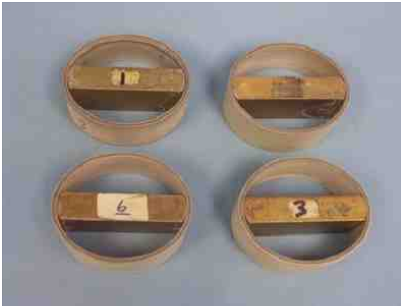
Figure 5 - Sn-Zn alloy plated 2a rings with stress bars inserted.
