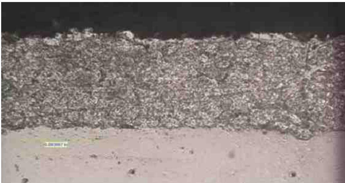
Figure 7 - Cross section of the tin-zinc alloy coating on a steel substrate.
