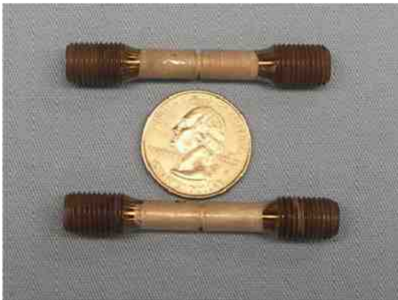
Figure 6 - Sn-Zn alloy plated 1a.1 notched bars after 200 hr of HE testing.
