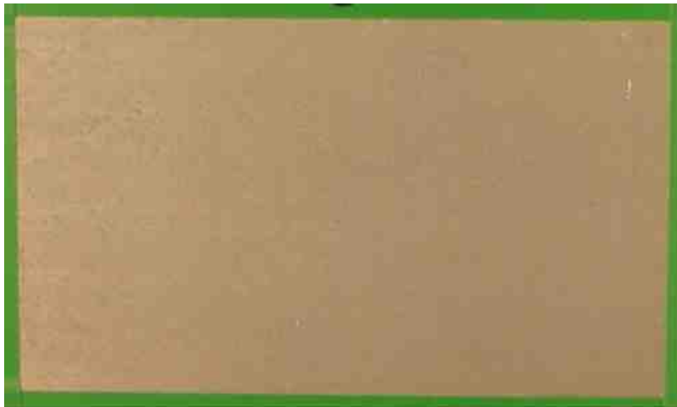
Figure 9 - Steel panel with a tin-zinc alloy coating and a chromium-free conversion coating after 96 hr of salt spray testing.
