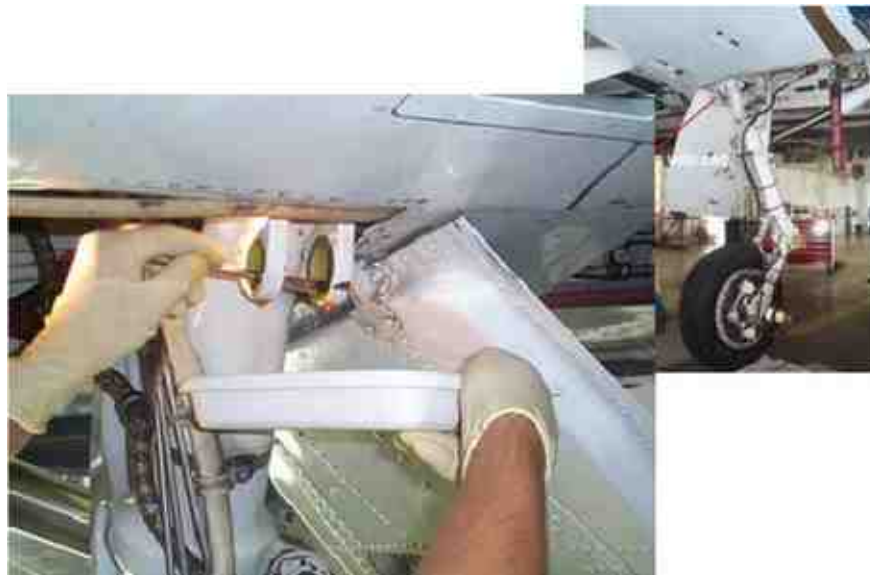
Figure 1 - Conversion coating being applied to a sacrificial coating brush plated onto a main landing gear bushing.
