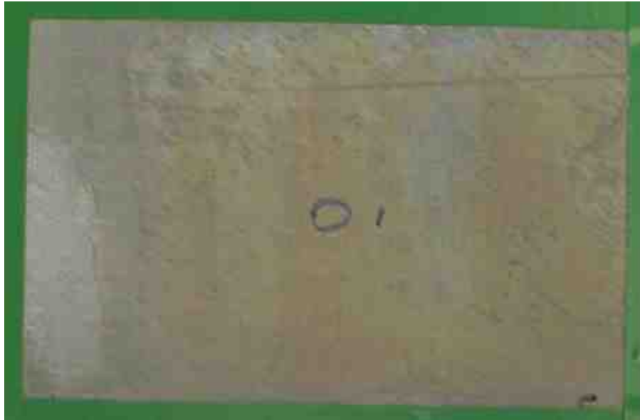
Figure 8 - Steel panel with a tin-zinc alloy coating and a trivalent chromium conversion coating after 96 hr of salt spray testing.
