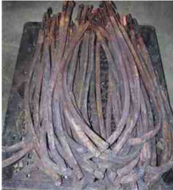
Figure 5 - Lead/tin anodes bent during plating.
