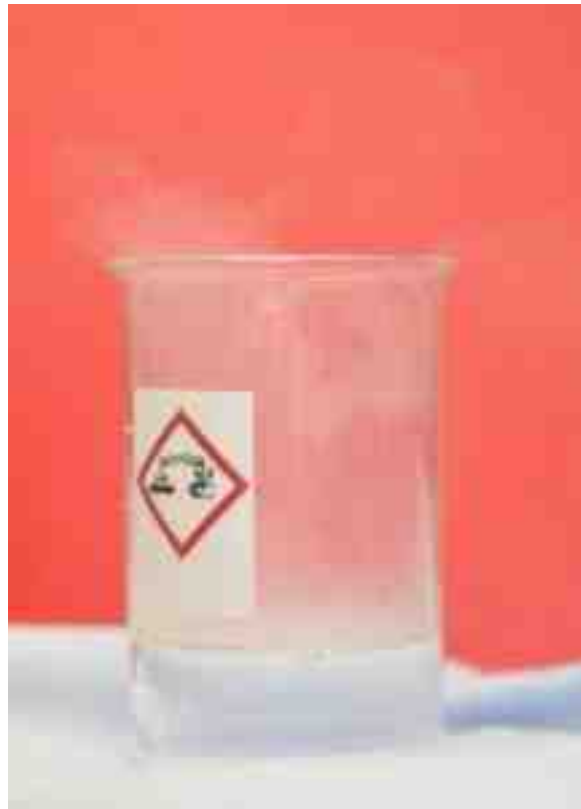
Figure 18 - Fumes after hydrochloric acid is added to water.
