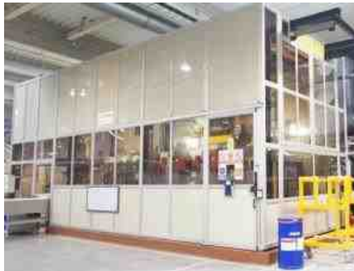
Figure 12 - A high productivity hard chromium plating line within a housing.
