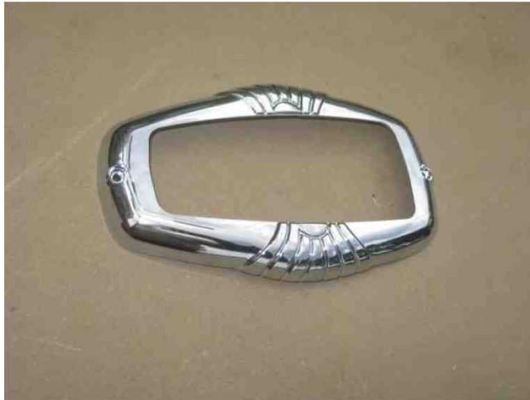
Figure 6 - An ABS component electroplated with Cu+Ni+Cr after palladium-free activation and electroless copper.
