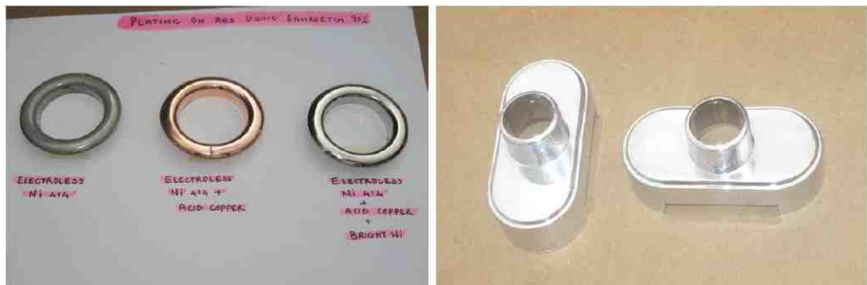
Figure 4 - The image on the left shows plated ABS ring pieces using the process sequence shown in Fig. 3: (L) after electroless Ni; (C) after electroless Ni + acid copper and (R) electroless Ni + acid Cu + bright Ni. The image on the right is of a Cu-Ni-Cr deposit on ABS components.
