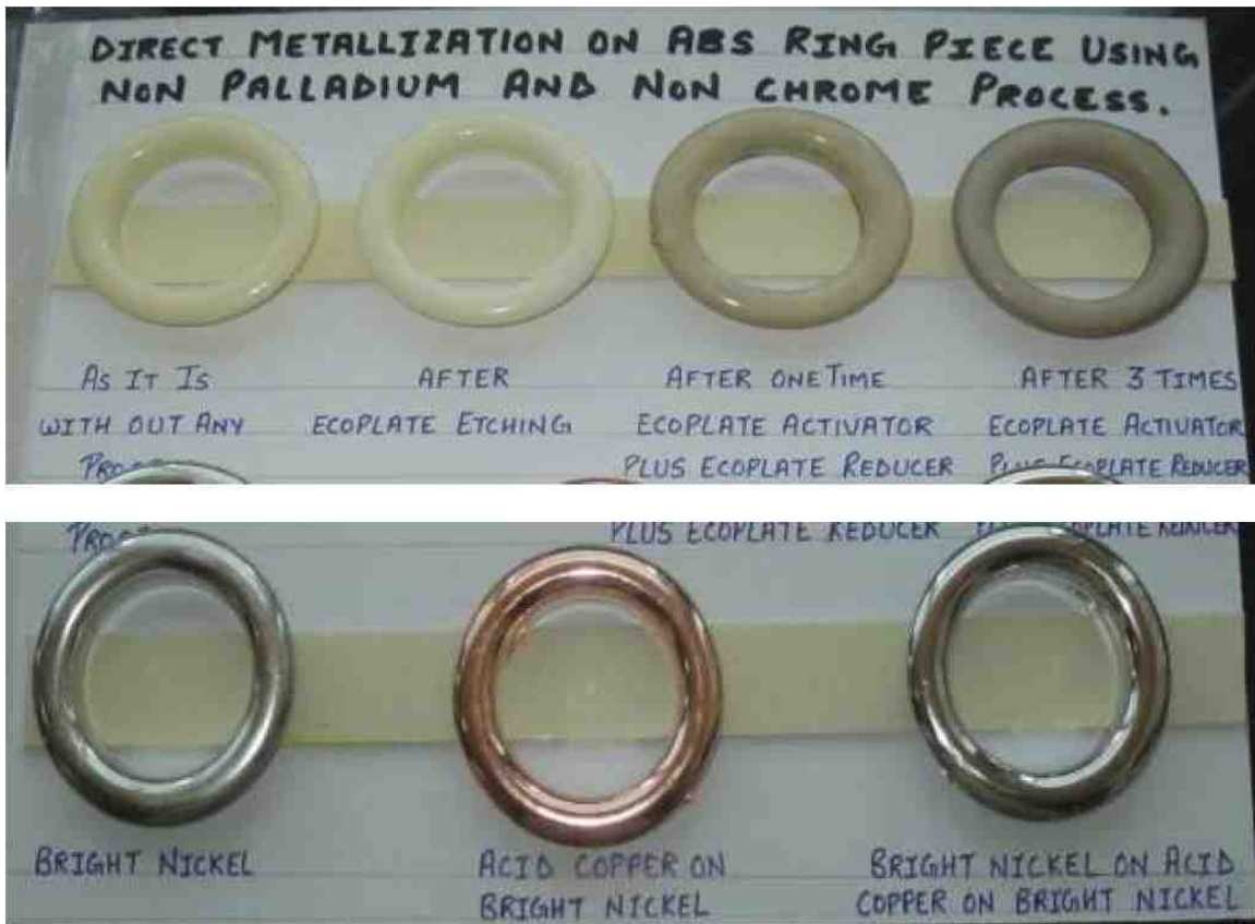
Figure 7 - Appearance of ABS pieces after each step in the ECOPLATE palladium-free activation process.
