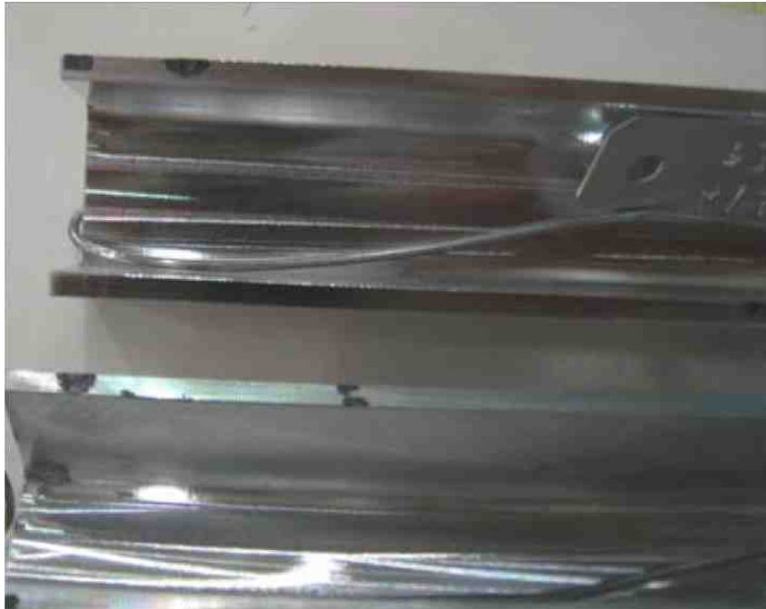
Figure 6 - Corrosion caused by alkaline degreaser with depleted silicates.
