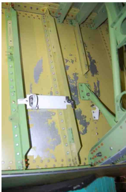
Figure 9 - Paint adhesion failure during assembly.
