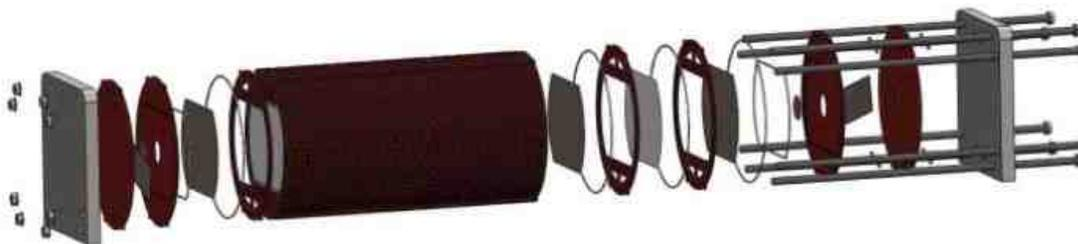
Figure 7 - CAD image of the construction of the electrolysis stack used for durability testing. Courtesy of GreenHydrogen.dk.
