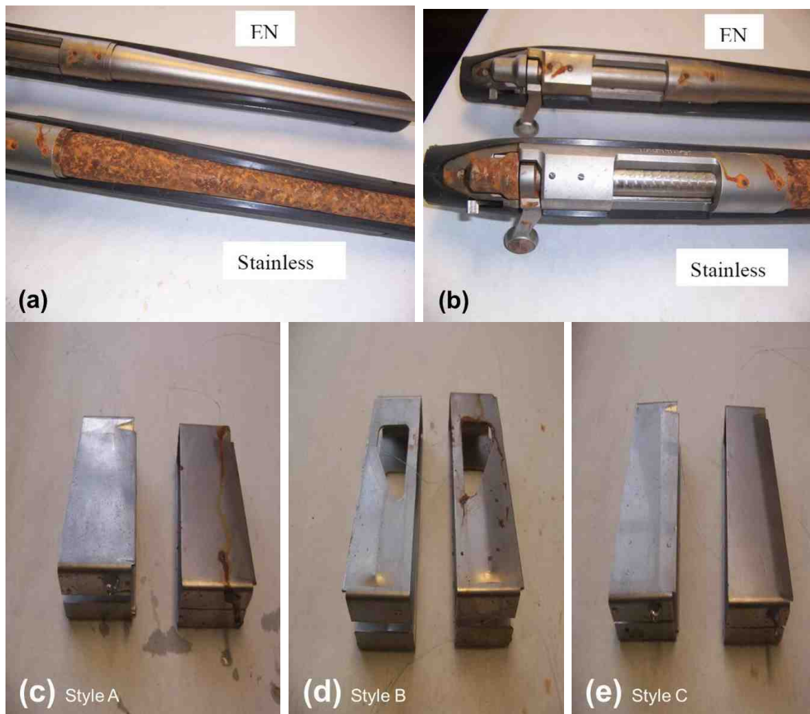
Figure 5 - Corrosion test results after 45 hours of salt spray: (a) barrels, (b) receivers, (c) magazine box style A, (d) magazine box style B and (e) magazine box style C. Both stainless (L) and electroless nickel (R) finishes are shown in each photo.
