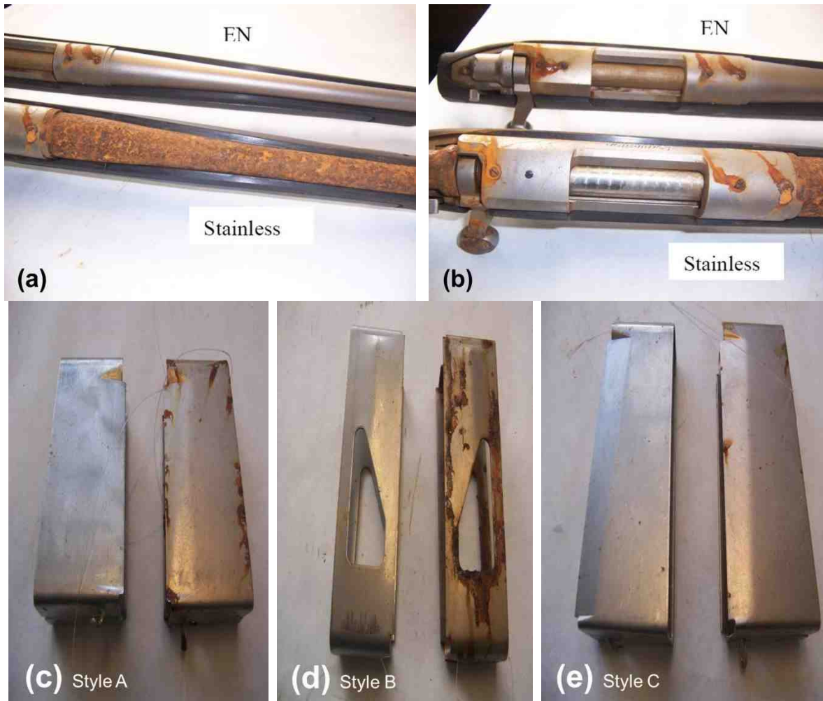
Figure 6 - Corrosion test results after 93 hours of salt spray at the end of the test: (a) barrels, (b) receivers, (c) magazine box style A, (d) magazine box style B and (e) magazine box style C. Both stainless (L) and electroless nickel (R) finishes are shown in each photo.
