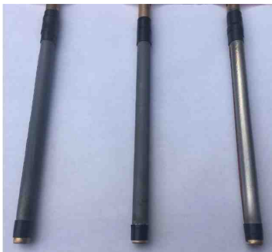
Figure 4 - Photographs of Ni-W-TiO 2 composite coatings plated with DC with no BD, PC with no BD, PC with 5mM BD (from left to right) on the rotating Hull cell.
