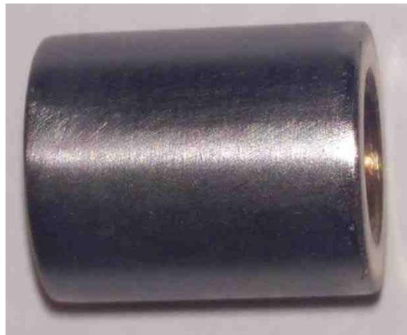
**Figure 7** - Optical image and photograph of 0.1M nickel-0.075M molybdenum deposit using an applied current density of 200 mA/cm<sup>2</sup>.
