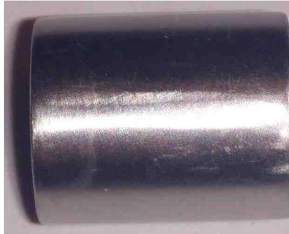
**Figure 6** - Optical image and photograph of 0.1M nickel-0.075M tungsten deposit using an applied current density of 50 mA/cm<sup>2</sup>.
