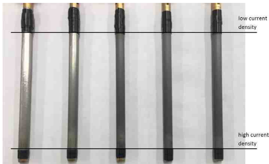
Figure 7 - Photographs of Ni-W deposits with 2.5, 7.5, 12.5, 25 and 50 g/L titania microparticles on the rotating Hull cell.
