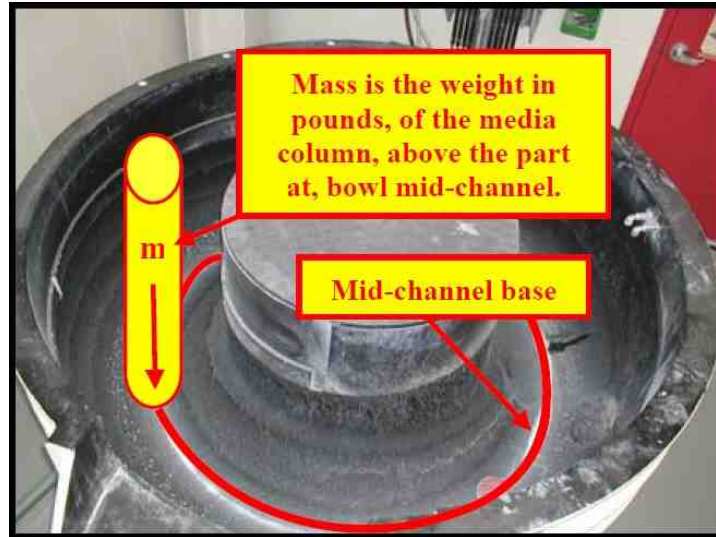
Figure 1 - Mass is the weight of the media column above a part at the bottom of the bowl at mid-channel.
