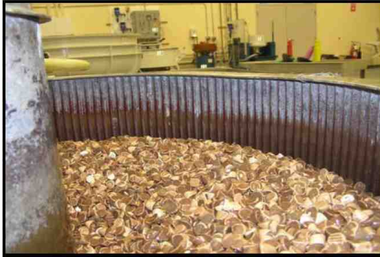
Figure 3 - Image of the same vibratory bowl where the media depth is too low, caused by attrition.
