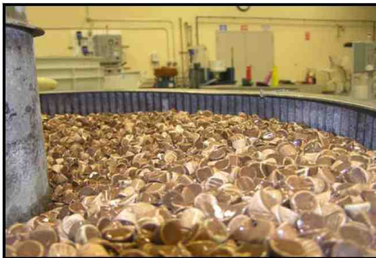
Figure 2 - Image of a vibratory bowl with the proper depth of media present in the bowl channel. 6
