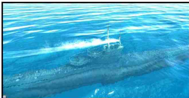
Figure 4 - A submarine near the surface has little water mass above its hull because the column of water above the submarine is virtually non-existent. 2
