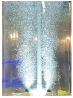
bar throughout the length of a tank. And lastly, pumped agitation with eductor nozzles, which is the focus of this paper.
