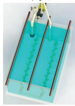
folds. The manifolds we design can also help to eliminate the buildup you tend to see around your heating elements or your anode bags.
